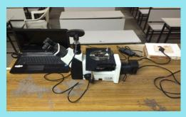
Motorized Stage Metallurgical Microscope
